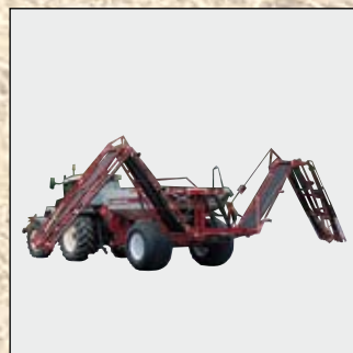
Hydraulic folding is standard on all booms.
