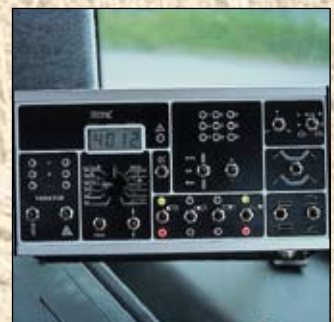
Tronic system enables to adjust the feed-rate from tractor cabin.
