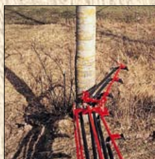
The outer section is fitted with a spring-loaded safety breakback.
