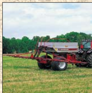
The hopper can be extended to 6000 litres.
